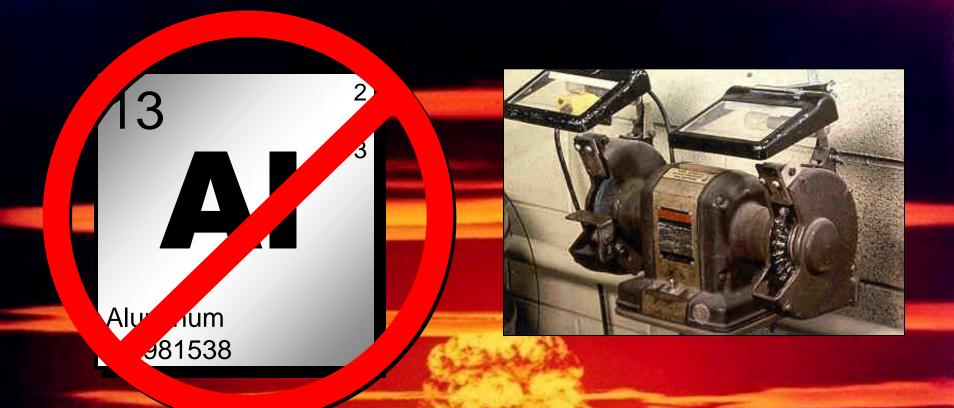
First and foremost, never use the grinding wheel to grind soft material like aluminum. Soft materials will coat the wheel and could cause excessive heat and even an explosion.
