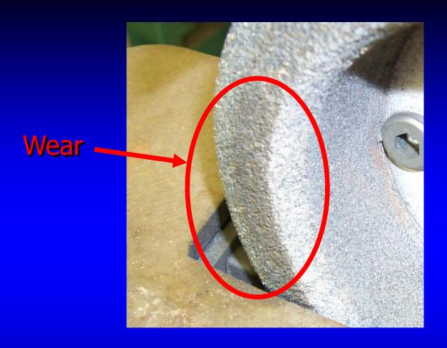
Check the grinding wheel before use for cracks or signs of wear. A worn grinding wheel will have an uneven grain, and should be dressed before use.
