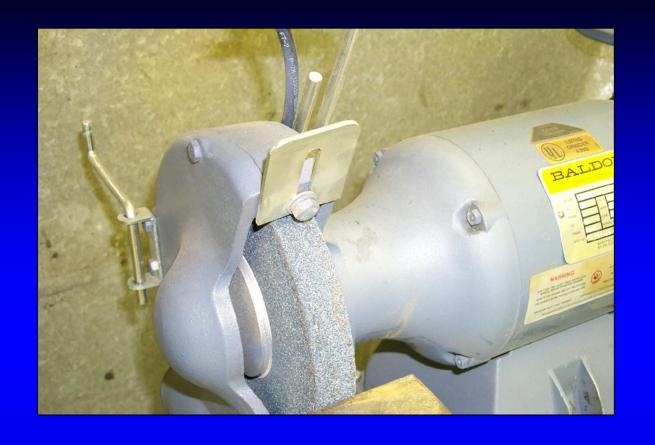
The primary purpose of a grinding wheel is to sharpen tools (e.g. drill bits). The hard abrasive wheel is made for removing very hard materials like high speed steel.
