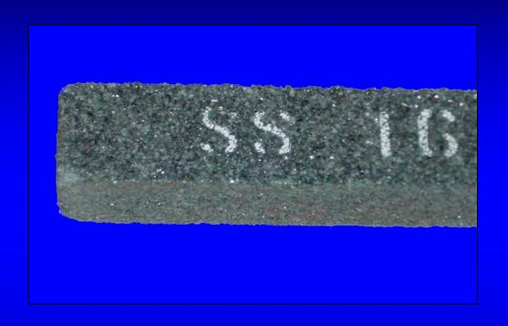
You can dress the wheel by grinding a block of carborundum across the surface of the wheel. This will even out the grain and remove excess material.
