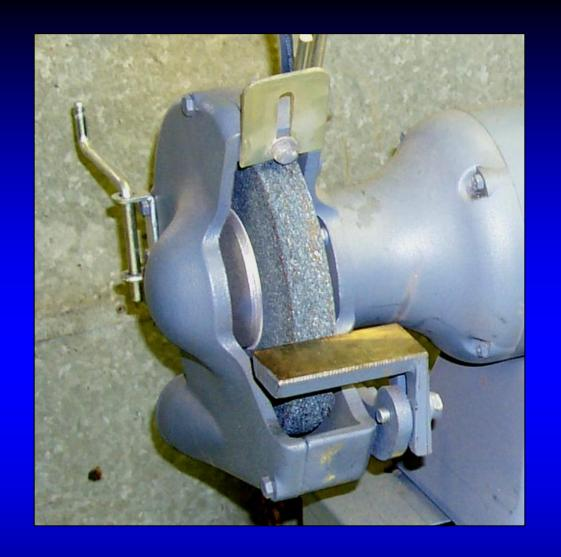
Q: This grinding wheel is coated with material. Can it be used in this condition?
