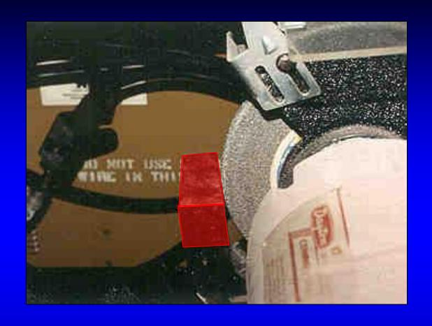
The tool rest should be set no more than 1/16" distance from the wheel for safe grinding.
