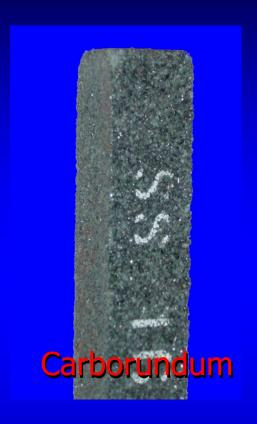
A: No! This wheel should be dressed by grinding a block of carborundum to remove the excess material before it can be used.
