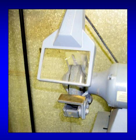
**Every grinding wheel** should be equipped with a glass guard. Look through the glass guard and not around it. If the guard is dirty, clean or replace it. Never use a grinder if its guard is off.
